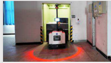
Elevator Transfer Between Floors
