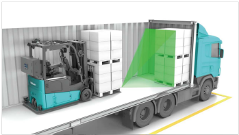
Automatic Check for Remaining Cargo on Trucks
