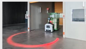
Elevator Transfer Between Floors
